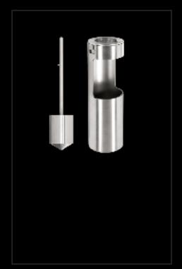
This measuring system owns two coaxial cylinders and it could be determine easily the dynamic viscosity and the yield value at 300 and 600 rpm, according A.P.I. standard, on drilling fluids, it could be also mesure the "gel" value at 3 rpm. It could equipped RM 100 and RM 200 RHEOMAT and also the portative viscometer RM 100 P.
