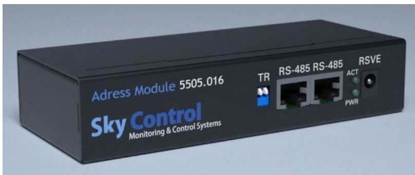
Pic. 5.7: Dry contacts unit 5505.016, front view
