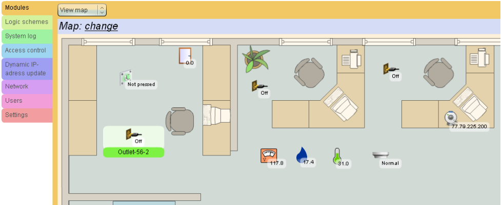
Pic. 2.13: Assigning sensor to location on a map
