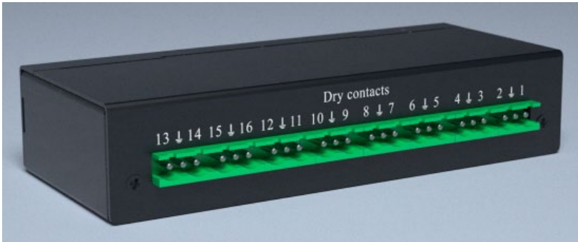
Pic. 5.9: Dry contacts unit 5505.016, back side
