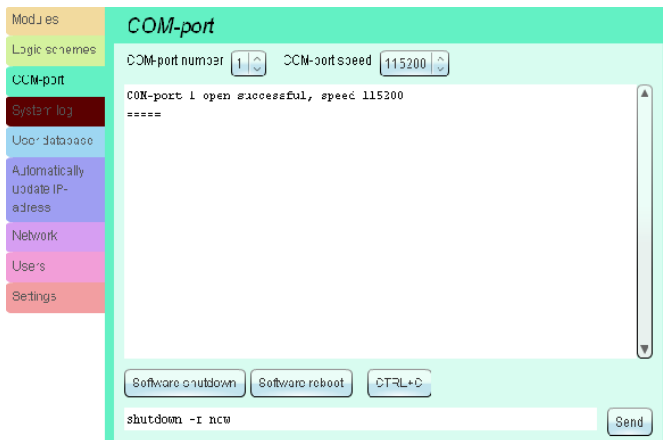
Pic. 2.19: COM-port remote control window
