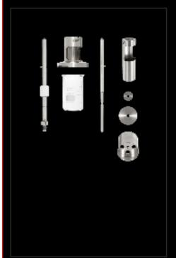
Stainless steel discs measuring system for viscosity measurements in a 150 ml Beaker.
