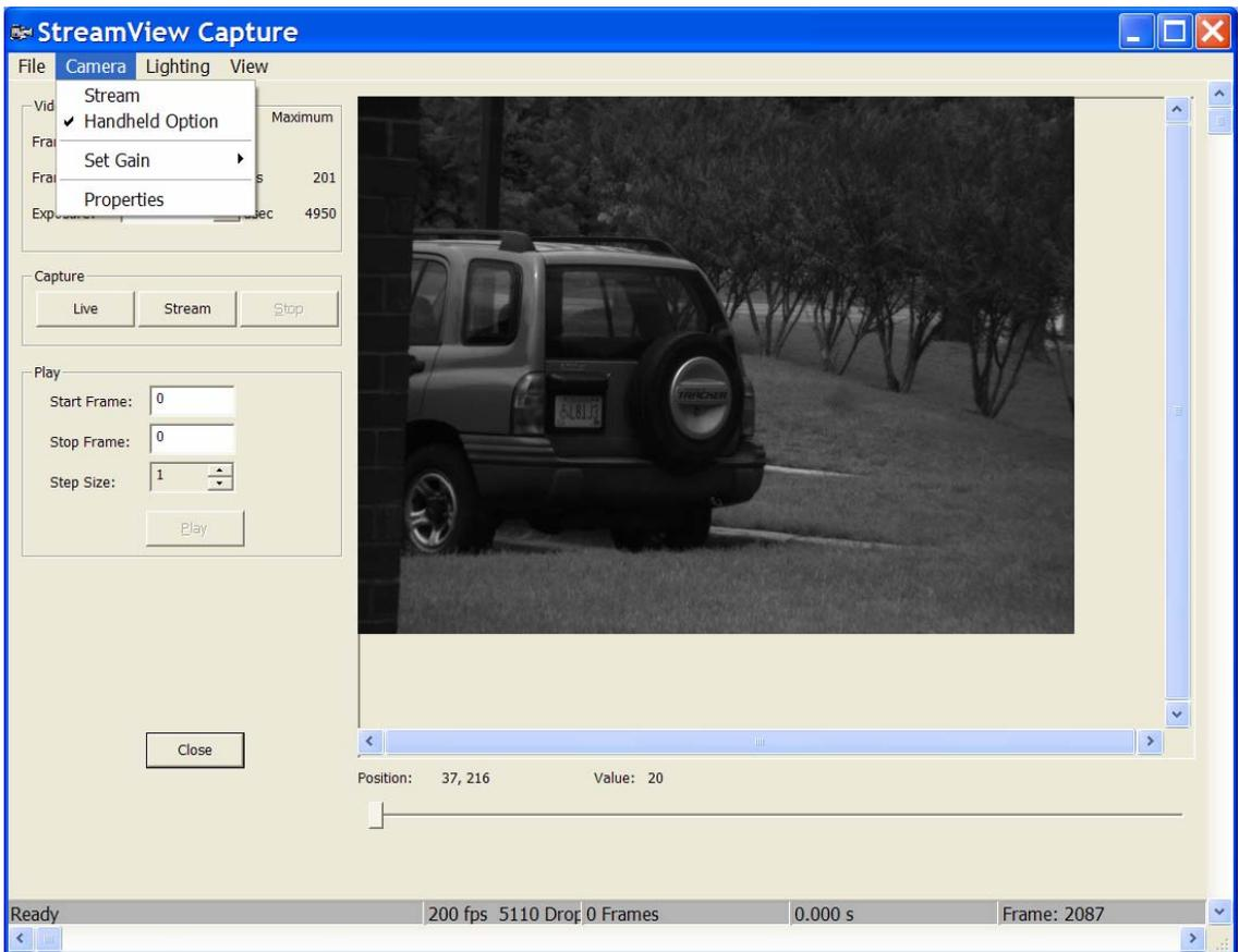
**Figure 20 Selecting [Handheld Option] for StreamView-LR Portable.**
