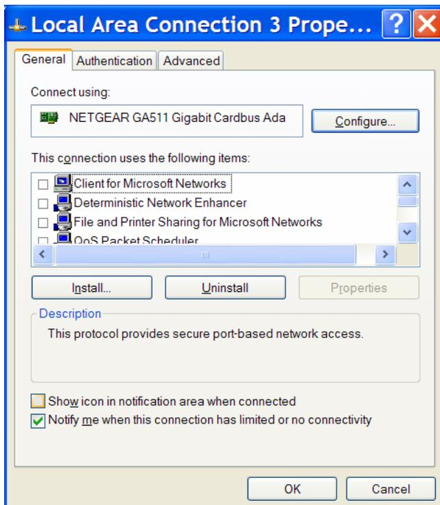
**Figure 6 Setting the network interface MTU size to match StreamView-LR.**
