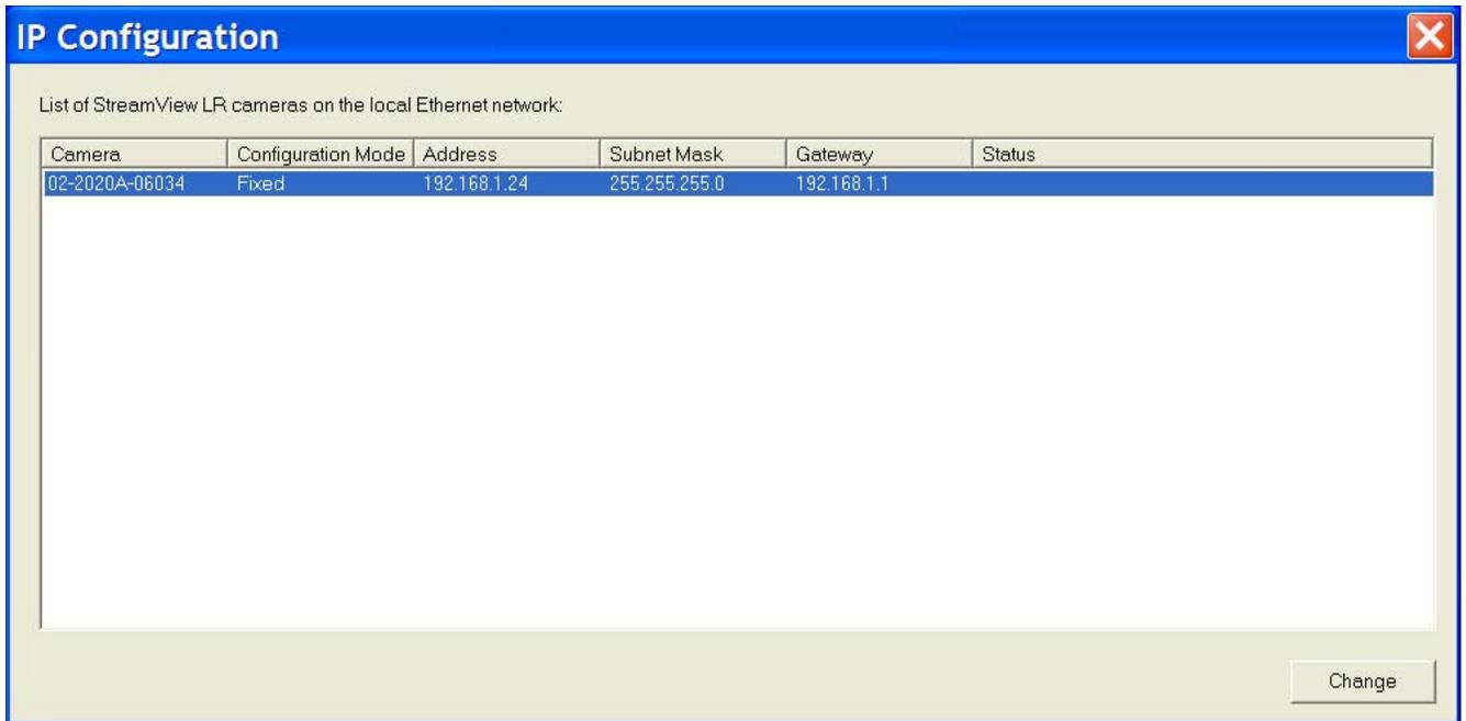
**Figure 2 StreamView-LR network configuration auto-discovery window.**
