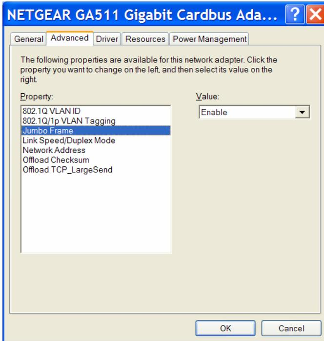
**Figure 7 Enabling jumbo frames on the network interface.**
